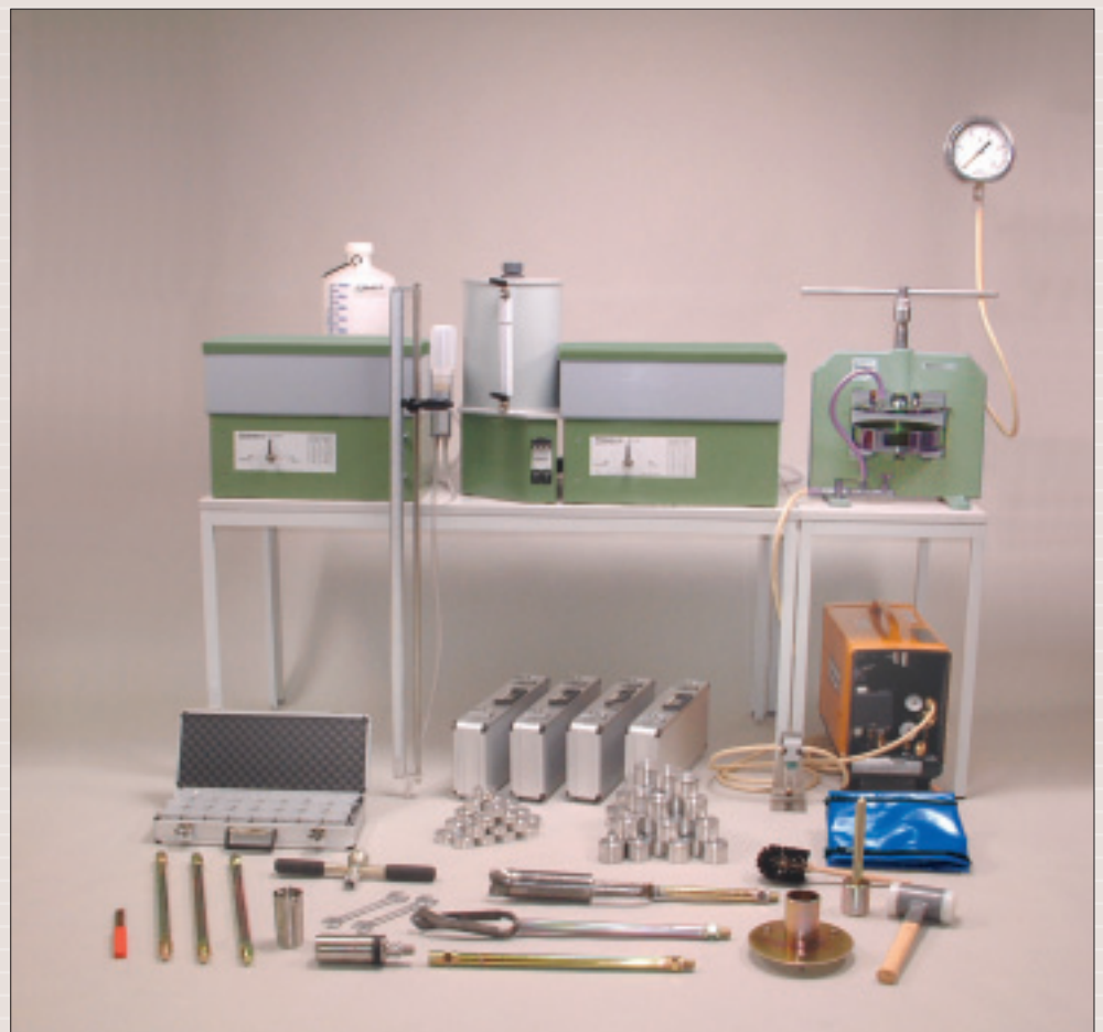
Set for pF determination, sandbox method (pF 0 - 4.2)
